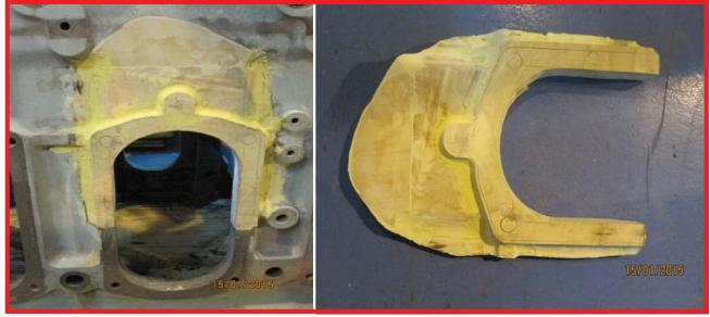
Material of the original block analyzed to determine the components. After getting analyse results proper material prepared to be used for casting. Patch fabrication by casting from determined material got completed.
