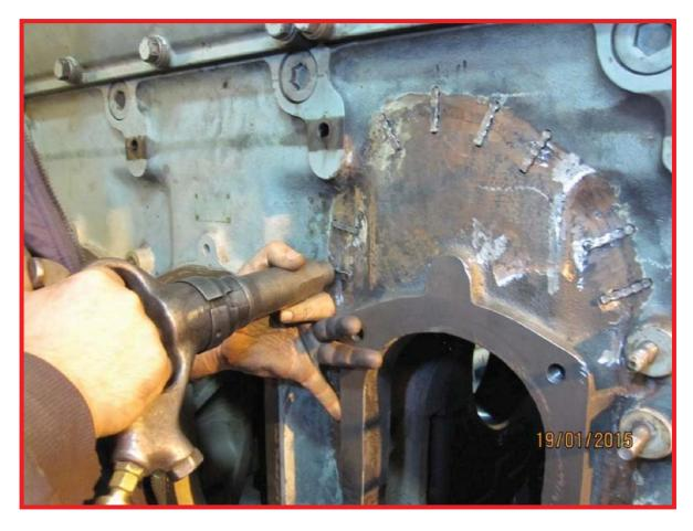
Finally upon completion of metalock repair grinding and surface dressing completed. Seat cover of the repaired part got flattened and holes drilled to be threaded for cover connection.
