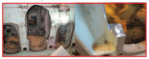
Upon completion cleaning and grinding of damaged surface modelling started. A model from wood manufactured carefully.
