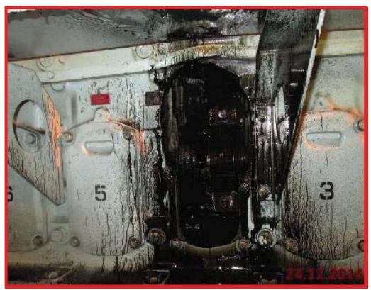
Cleaning and preperation of the damaged area completed. Thin walls removed by grinding
