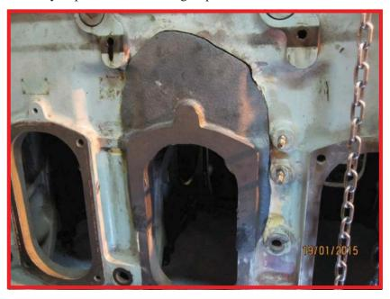
Once alignment of the fabricated casting finished standart metalock repair followed to conclude the repair
